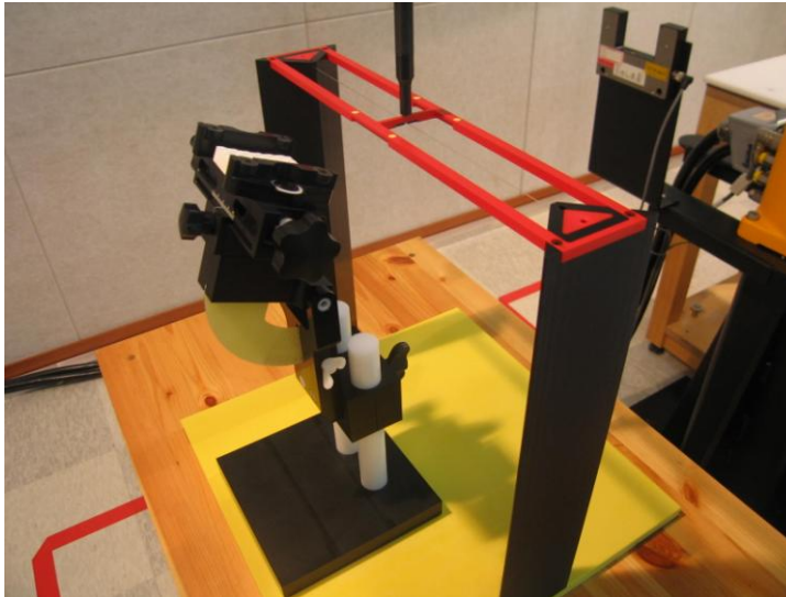
Figure 2. HAC Phantom & Device Holder
