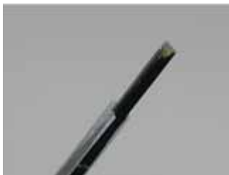
Figure 6. EX3DV4 E-field Probe
