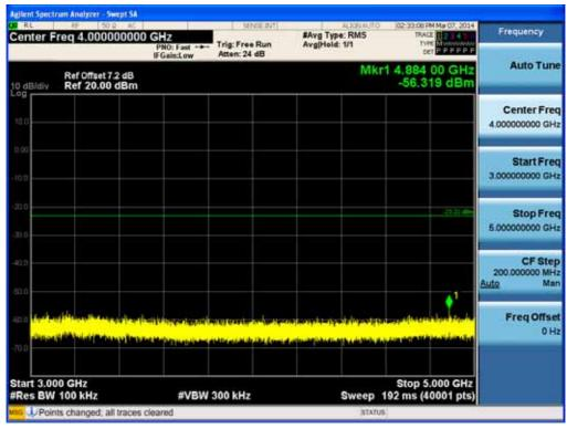
Test Plots (8DPSK) - 5 GHz - 7 GHz Spurious Emission (Low-CH)
