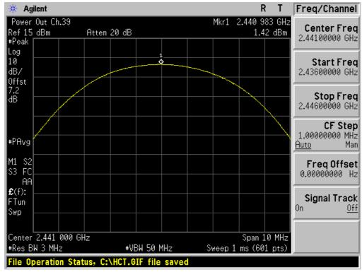
Test Plots (8DPSK) Peak Power (High-CH)
