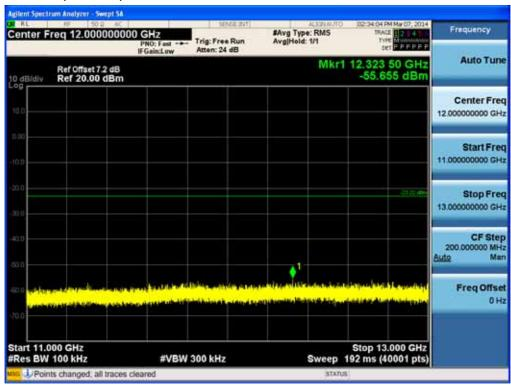
Test Plots (8DPSK) - 13 GHz – 15 GHz Spurious Emission (Low-CH)
