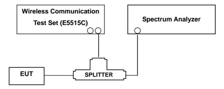
(Configuration of conducted Emission measurement)
