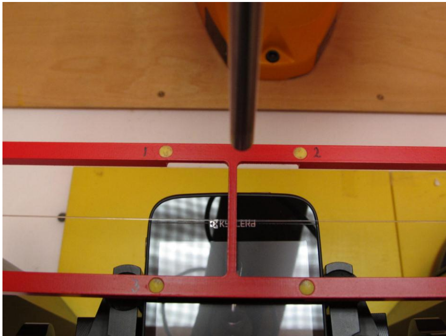
Figure 1b – HAC Tcoil Emission Test Setup
