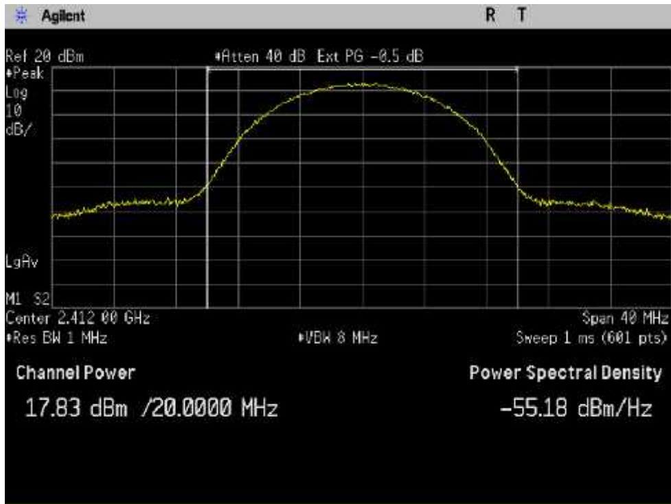
Figure 7-1: Output Power 802.11b, 11Mbps, Ch 1
