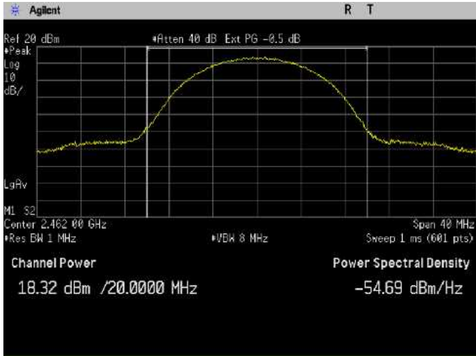
Figure 7-3: Output Power 802.11b, 11Mbps, Ch 11
