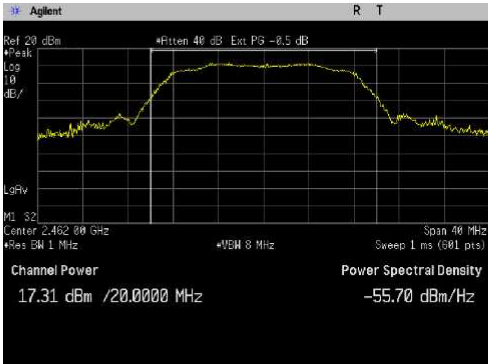
Figure 7-6: Output Power 802.11g, 6 Mbps, Ch 11
