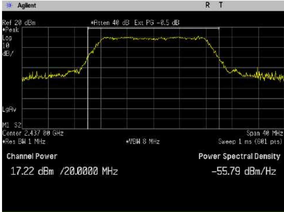
Figure 7-5: Output Power 802.11g, 6Mbps, Ch 6
