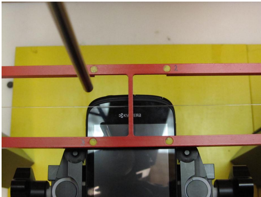
Figure 1b – HAC T-Coil Test Setup
