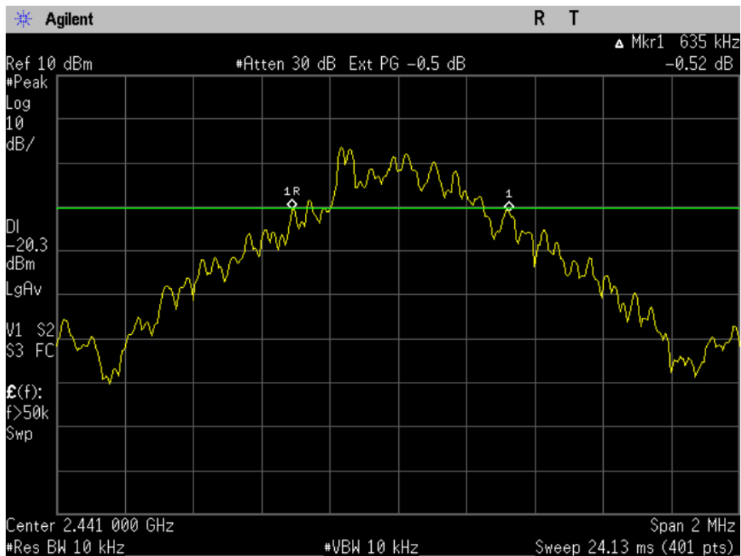
Figure 6-2a: 20dB Bandwidth Basic rate, Channel 39.
