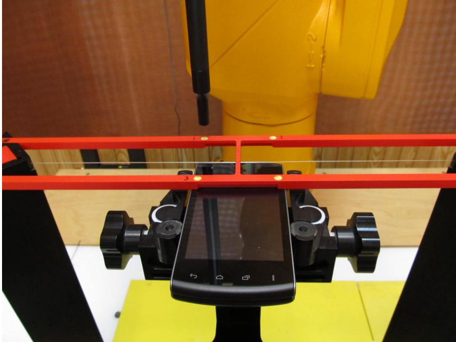
Figure 1a – HAC RF Emission Test Setup
