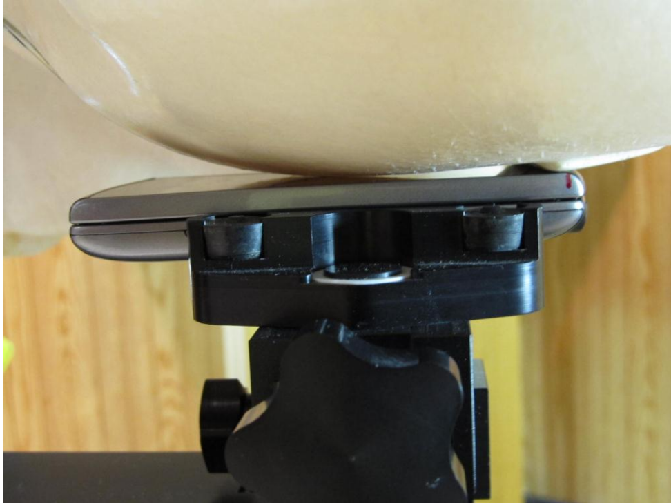
Figure 9E.1 Phone Closed against the head (Left cheek position)
