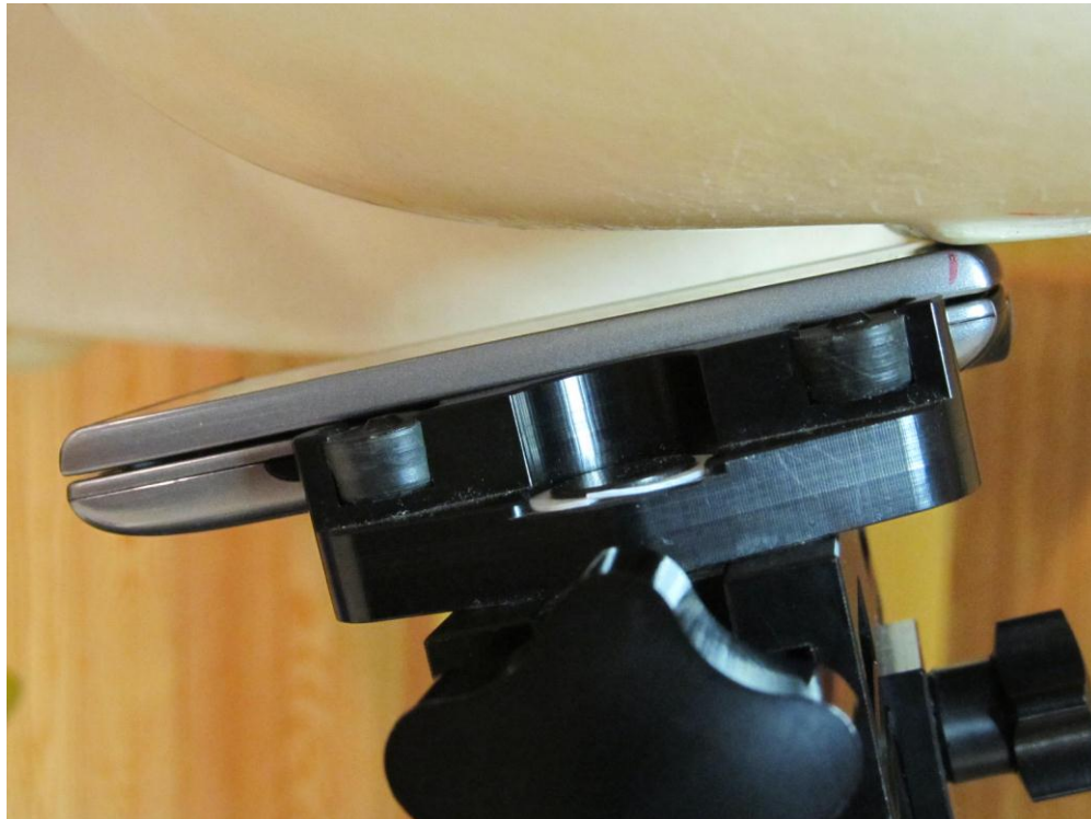
Figure 9E.1 Phone Closed against the head (Left cheek position)
