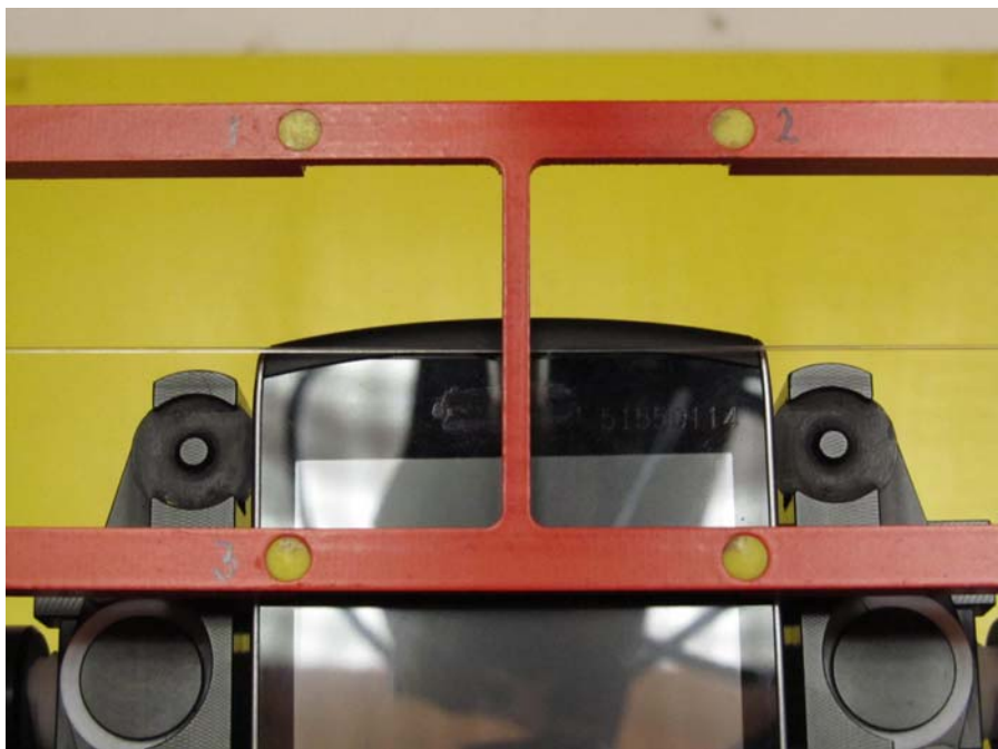
Figure 1b – HAC RF Emission Test Setup
