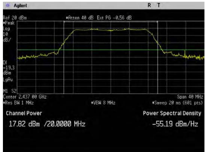
Figure 7-5: Output Power 802.11g, 6Mbps, Ch 6
