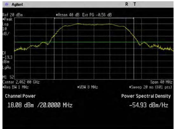
Figure 7-6: Output Power 802.11g, 6 Mbps, Ch 11
