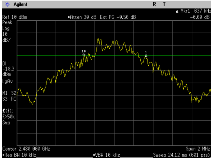
Figure 6-3a: 20dB Bandwidth Basic rate, Channel 78.
