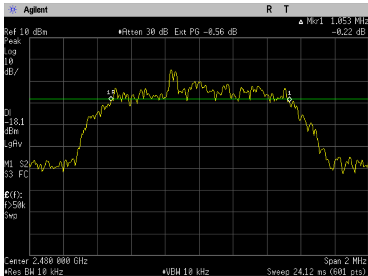
Figure 6-3b: 20dB Bandwidth EDR DQPSK, Channel 78.
