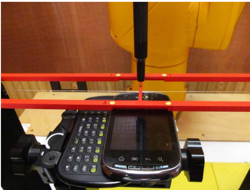
Figure 1b – HAC RF Emission Test Setup, Slide Open
