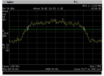
Figure 6-3c: 20dB Bandwidth EDR D8PSK, Channel 78.
