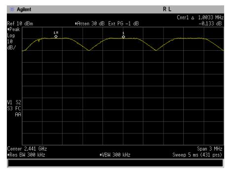
Figure 7: Carrier Frequency Separation between channels 38, 39 (mid-channel) & 40.
