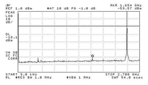
Figure 11-1a: Conducted Spurious Emissions (CH 0).
