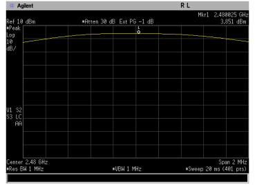
Figure 5-3b: Peak Output Power, EDR D8PSK Channel 78.
