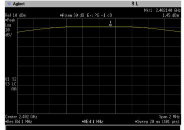
Figure 5-1a: Peak Output Power, EDR DQPSK Channel 0.
