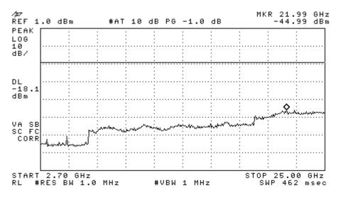
Figure 11-1b: Conducted Spurious Emissions (CH 0).
