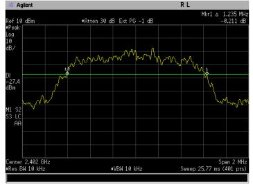
Figure 6-1c: 20dB Bandwidth EDR D8PSK, Channel 0.
