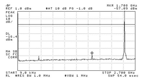
Figure 11-2a: Conducted Spurious Emissions (CH 39).
