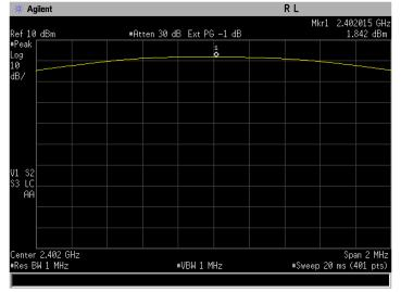
Figure 5-1b: Peak Output Power, EDR D8PSK Channel 0.
