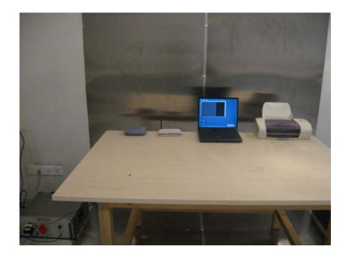
Radiation Emission Test Setup (30MHz to 1GHz)
