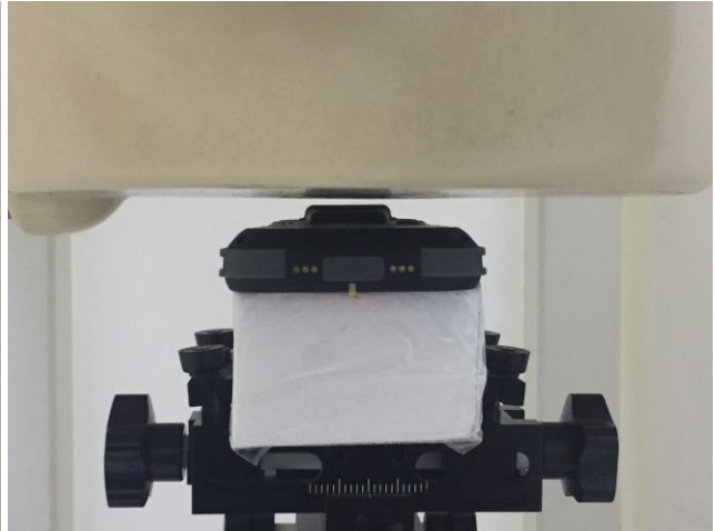
Back, Test Separation 10 mm for WWAN
