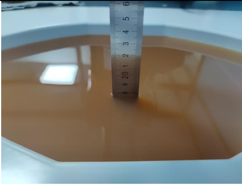
Fig. 9.1 Photo of Liquid Height for Extremity SAR (depth>15cm)
