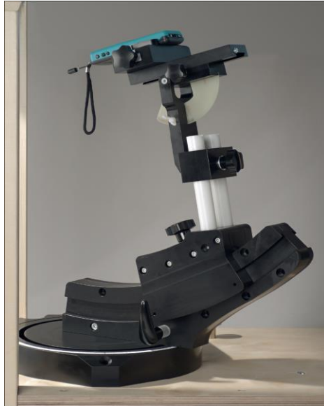
F-2. Device Holder for Transmitters
