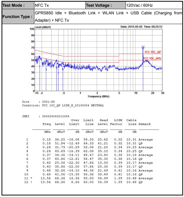
(1) The EUT is with NFC antenna during testing.
