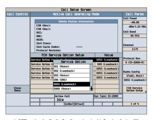
1xRTT setting for Radio Configuration 1 with Service Option 55
