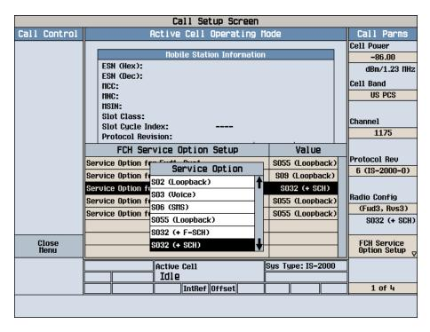
1xRTT setting for Radio Configuration 3 with Service Option 32
