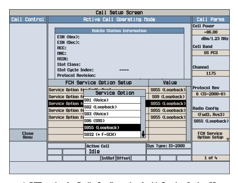
1xRTT setting for Radio Configuration 3 with Service Option 55
