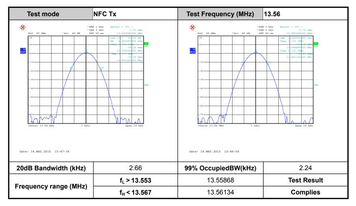
C.1 Test Result of 20dB Spectrum Bandwidth
