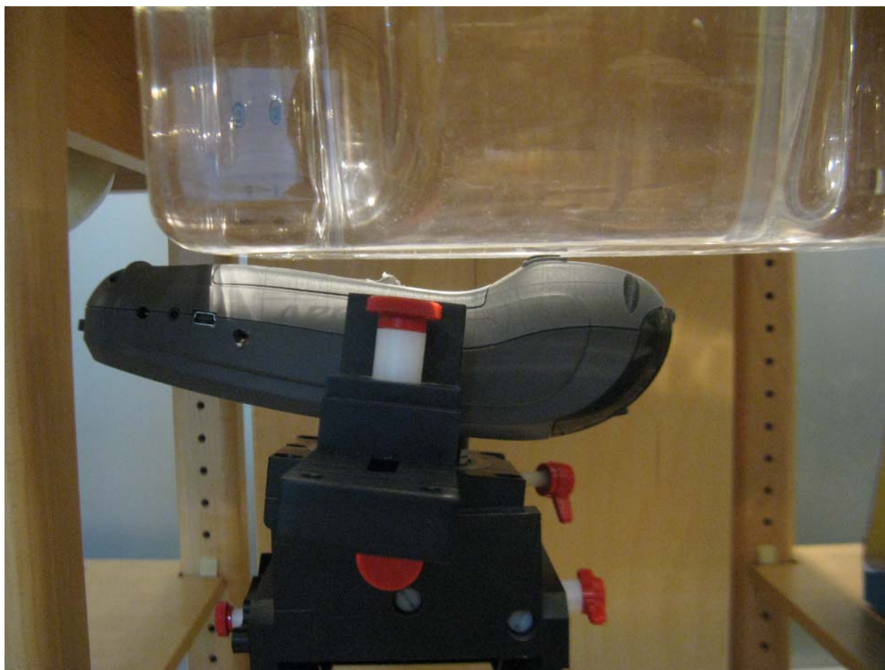
Body-worn Setup Photo (Back touching the flat phantom)
