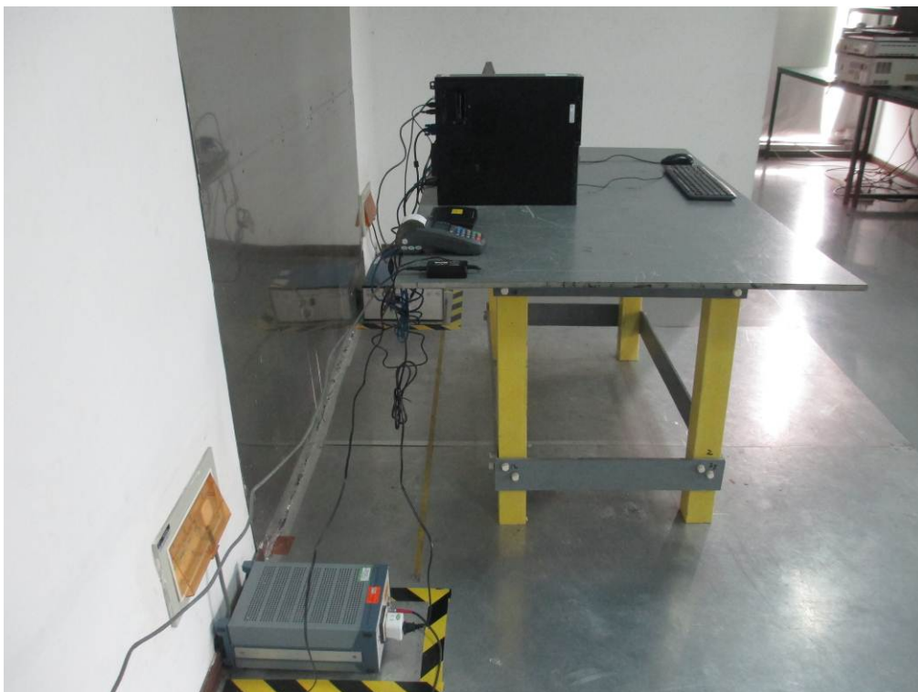
Conducted Emissions Test Setup Side View
