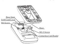
2) For SAM card installation, please refer to the following figure: ①Open up SAM card cover, which is at the bottom of the terminal; @Put SAM card into corresponding SAM card slot; ③Put SAM card cover back.
