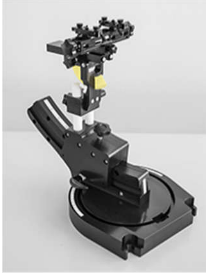
Mounting Device for Hand-Held Transmitters
