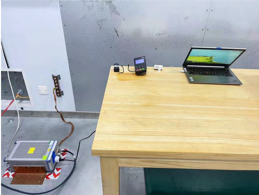
AC Power Line Conducted Emission
