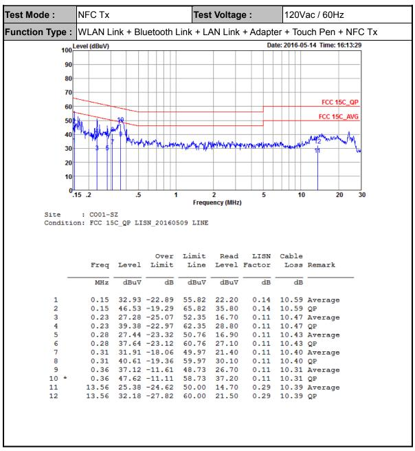
(2) The NFC antenna is replaced by a dummy load during test.
