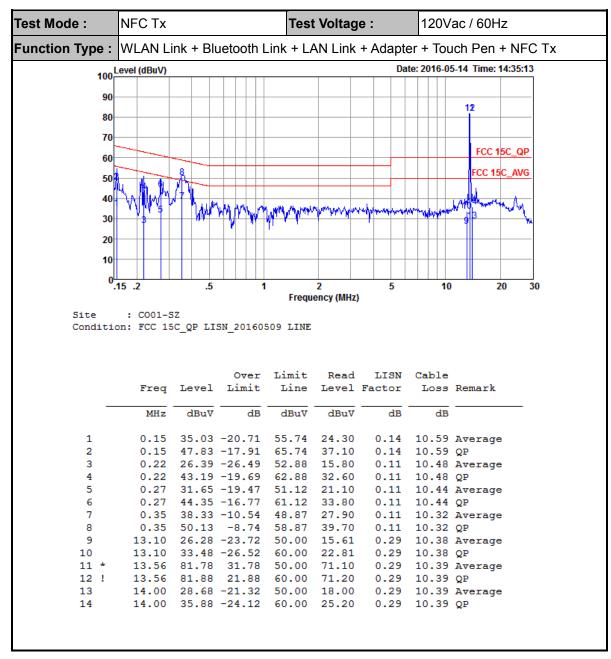
(1) The EUT is with NFC antenna during testing.
