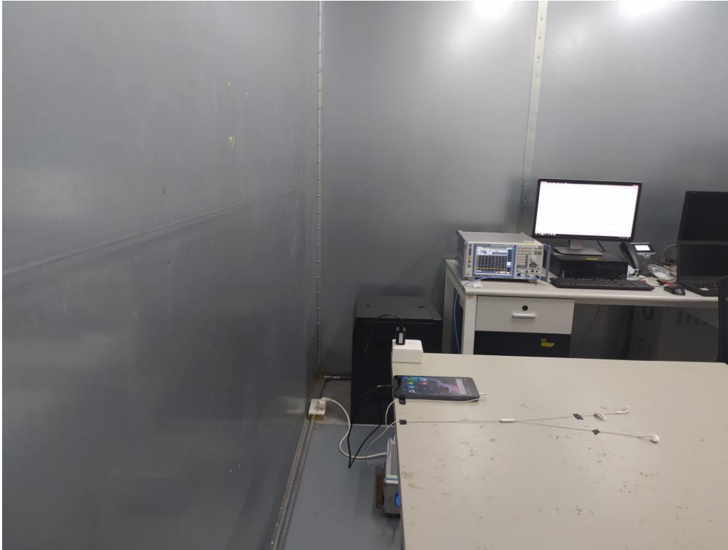
Fig. 3 Power line conducted emission setup photo
