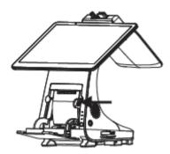
3. Open the built-in and external printer covers as shown in the figure.
