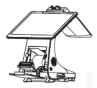
5. Close the printer covers in turn. The "Out of Paper" indicator will light off. The paper is changed successfully.
