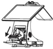
4. Load the paper roll and make sure a part of paper is exposed.
