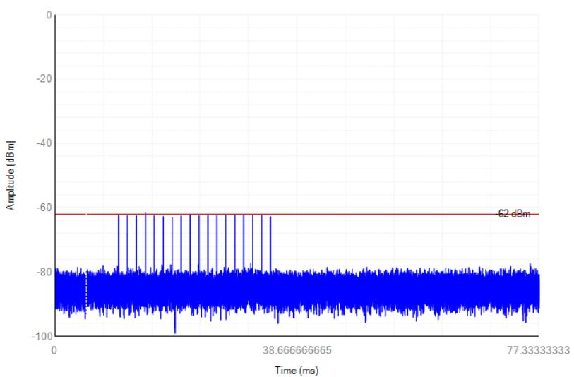
**Radar Type 0****802.11ac80: 5530MHz****Radar Calibration**
