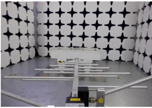
Transmitter Radiated Unwanted Emissions(Above 1GHz)
