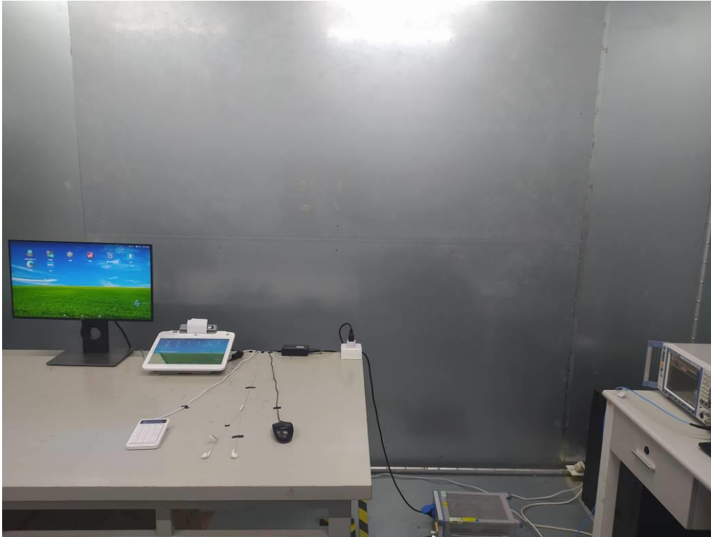
Fig. 3 Power line conducted emission setup photo
