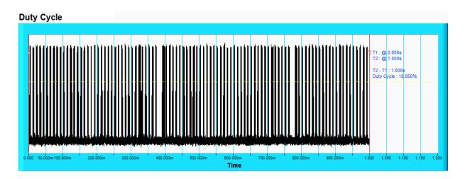
**NOTE**: T1 denotes the start of duty cycle period is 0th second. T2 denotes the end of duty cycle period is 1th second. T2 - T1 = 1 seconds. Duty Cycle = 18.856%.
