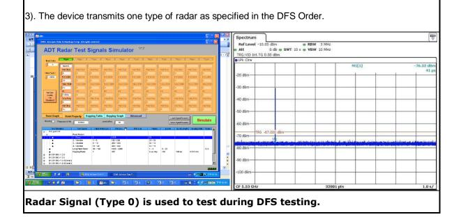
The test frequency has been monitored to ensure no transmission of any type has occurred for 30 minutes;
