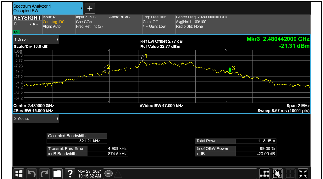
-20dB Bandwidth NVHT 2-DH1 2402MHz Ant1
