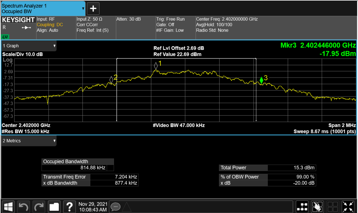
-20dB Bandwidth NVHT 1-DH1 2441MHz Ant1
