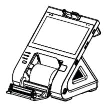
5. Close the Printer Cover as shown in the picture, and press the Printer Cover with both hands into the paper warehouse.
