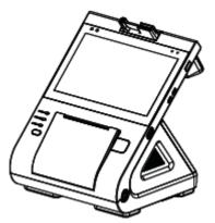
3.0pen the Printer Cover completely in the direction of the arrow.
