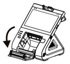
4.Load the paper roll as the picture shows, and left a sheet of paper to be exposed.
