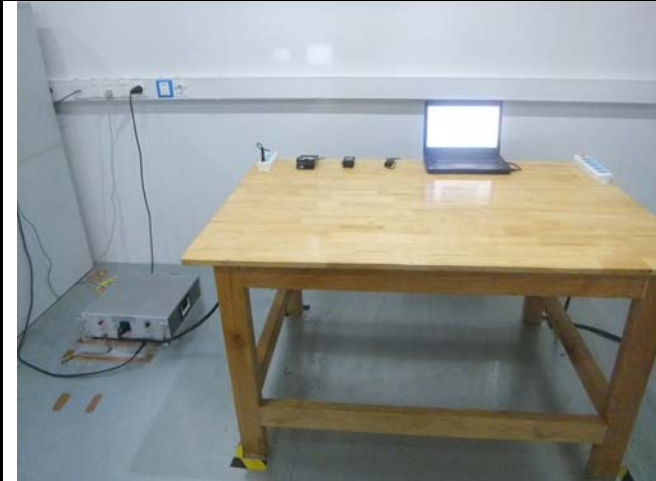
Conducted Emissions Test Setup Front View
