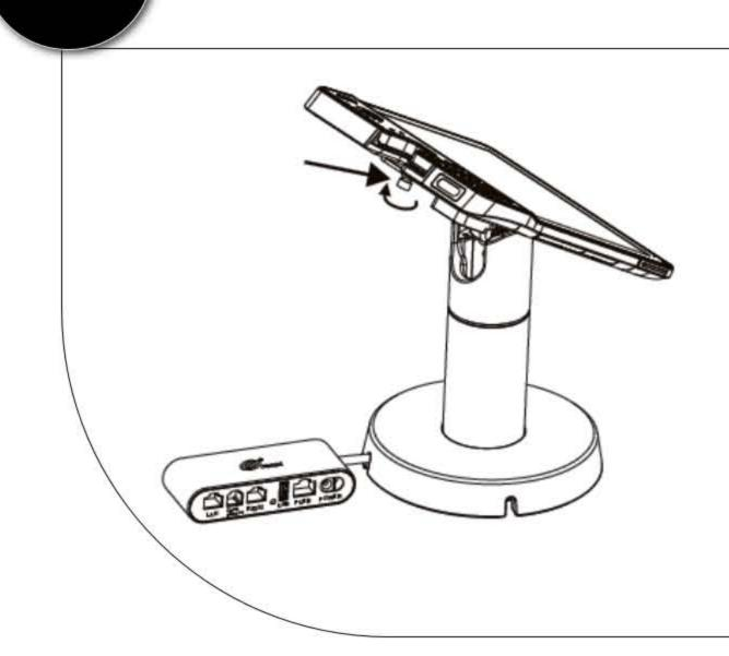
Loosen screws in a clockwise direction.
