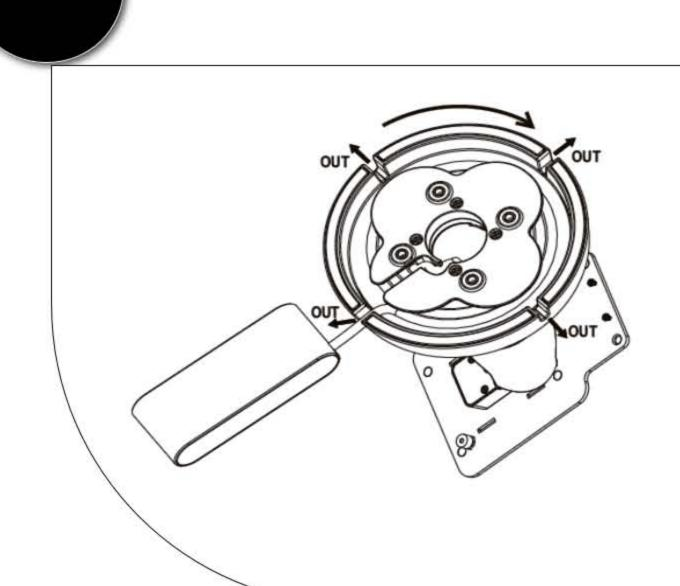
• There are four outlets on the underside of the base plate that are designed for different placement options for the communication box.
