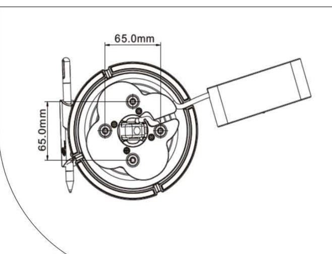
• Secure to countertop by drilling holes into cashier desk. Drill four holes in a circle at angles of 0°, 90°, 180°, and 270° with a 65mm space between the two horizontal holes, as shown
