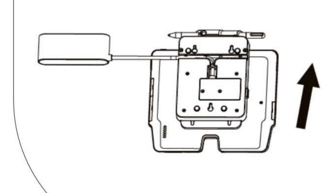
• Press and hold the orange button on the side of the plate to release the tablet. Slide the plate in the direction shown to remove it.
