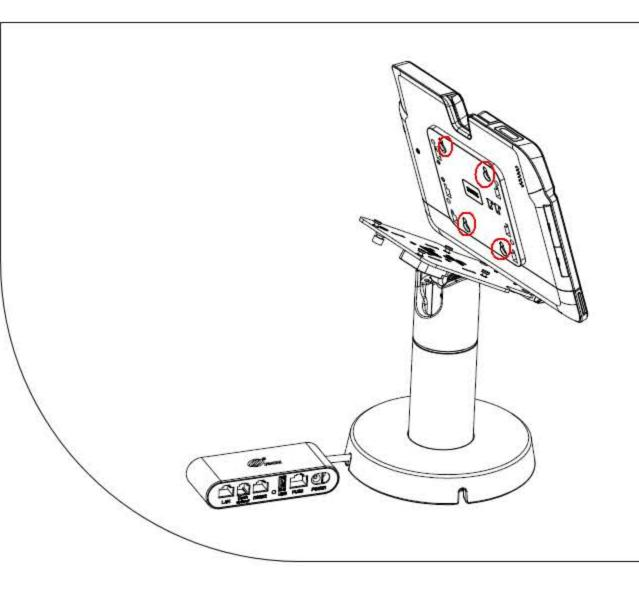
• Place tablet on stand, as shown, aligning the four holes on the underside of the tablet with the screws on the adapter.
