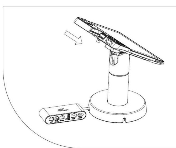
• Push tablet forward slightly, in the direction shown, so that it is firmly secured to the stand.
