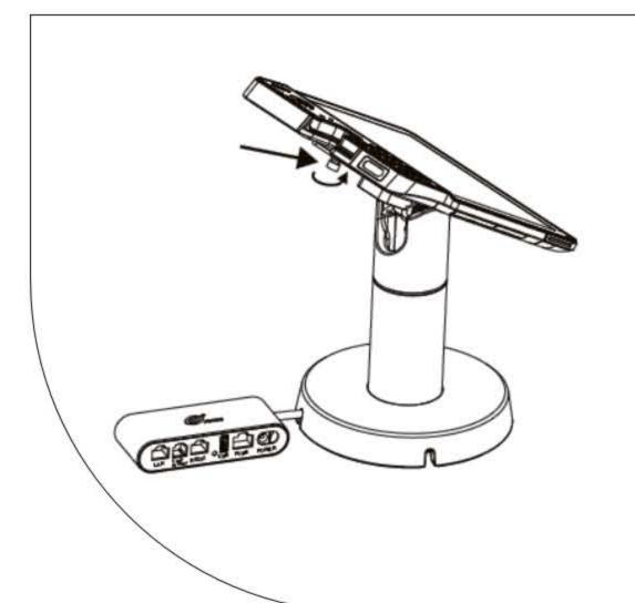
• Tighten the screw on the underside of the stand mounting plate in a counter clockwise direction.
