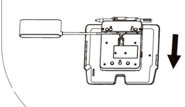
• Push plate in direction shown below to the end to lock it.
