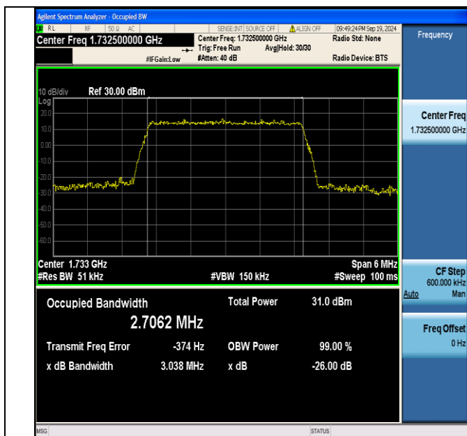
Band4-3MHz-16QAM-20175-15RB#0-PASS
