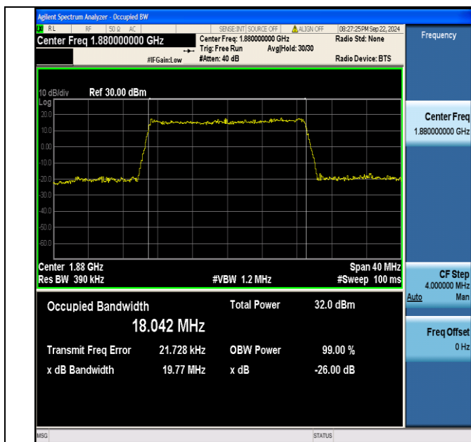
Band2-20MHz-16QAM-18900-100RB#0-PASS
