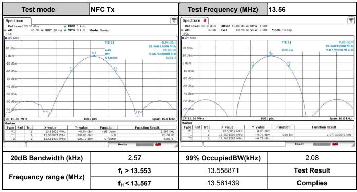
**Remark:** Because the measured signal is CW adjusting the RBW per C63.10 would not be practical since measured bandwidth will always follow the RBW and the result will be approximately twice the RBW.
