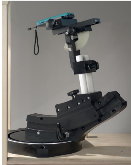
F-2. Device Holder for Transmitters
