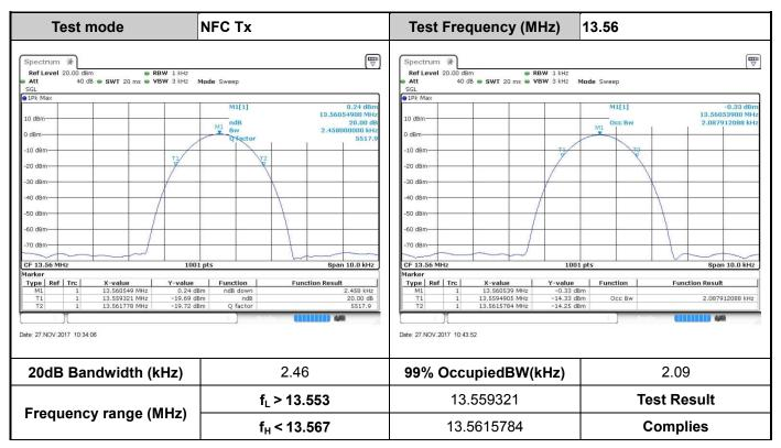
B1. Test Result of 20dB Bandwidth and 99% Occupied Bandwidth
