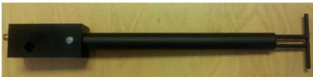
Figure 1 – MVG COMOSAR Validation Dipole
