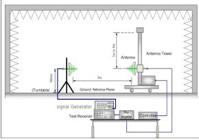
Test Setup for Above 1 GHz
