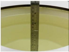
Fig 10.1 Photo of Liquid Height for Body SAR
