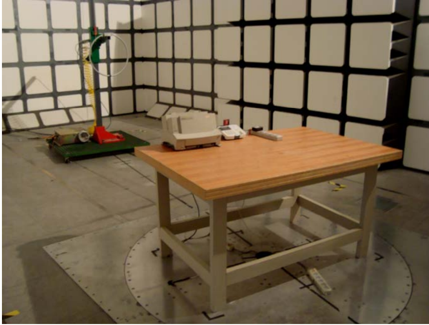
Below 30 MHz: Radiated Emissions - Rear View
