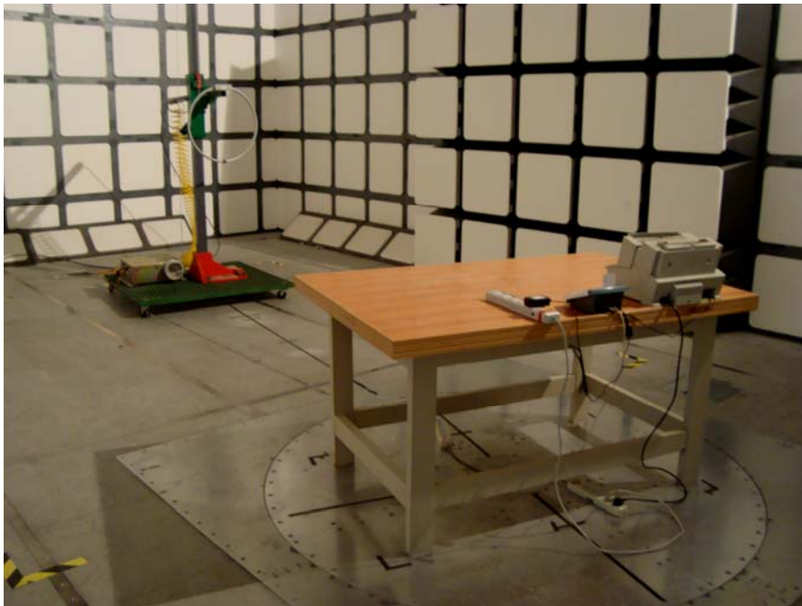
Below 30 MHz: Radiated Emissions - Rear View
