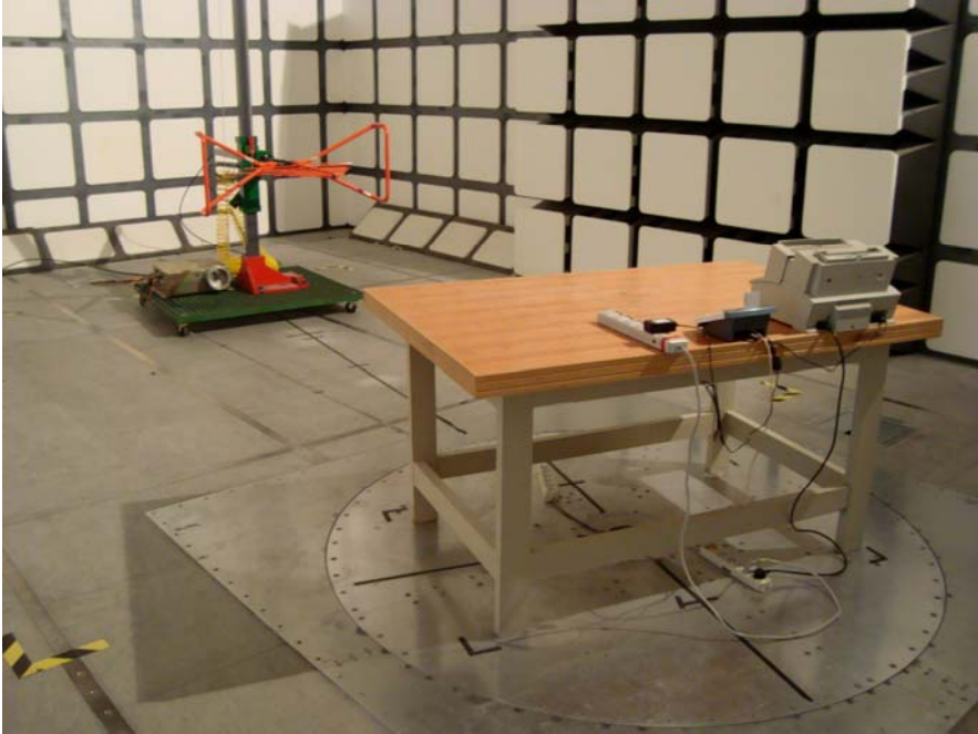
Above 30 MHz: Radiated Emissions - Rear View
