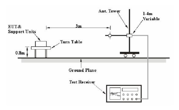
The radiated emission tests were performed in the 3-meter chamber A test site, using the setup accordance with the ANSI C63.4-2003. The specification used was the FCC Part Subpart C limits.
