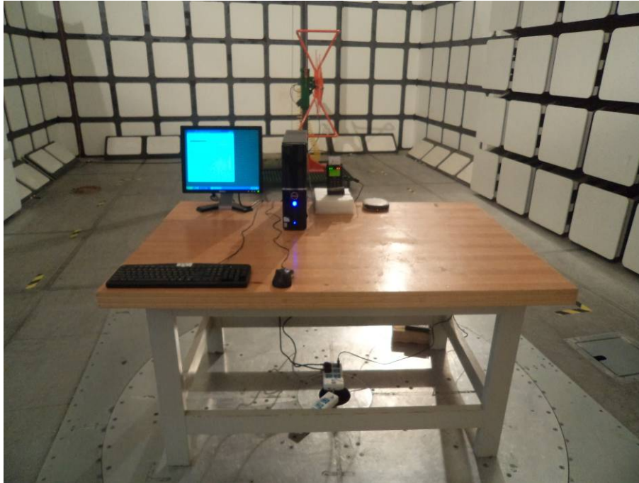
Radiated Emissions – Front View (Above 30 MHz) (PC-Linked)
