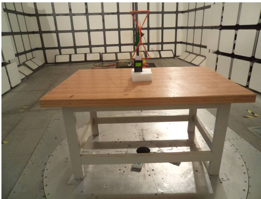
Radiated Emissions View (Above 30 MHz) (Stand-alone)
