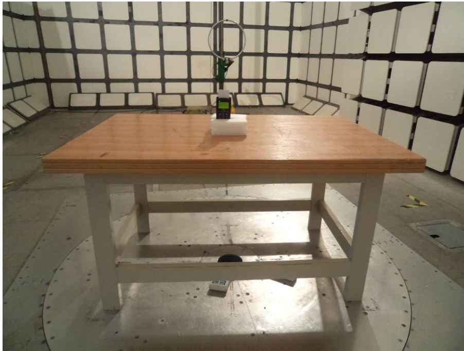
Radiated Emissions View (Below 30 MHz) (Stand-alone)
