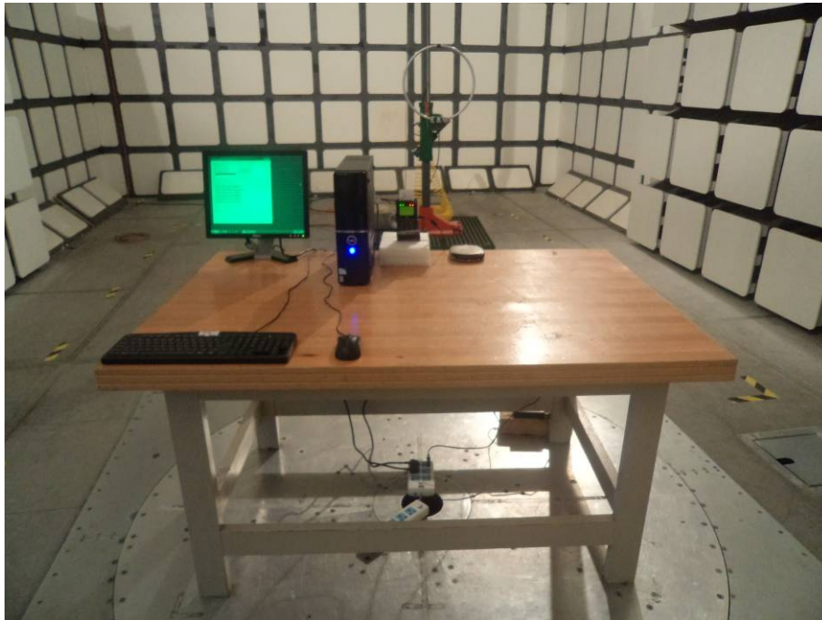
Radiated Emissions – Front View (Below 30 MHz) (PC-Linked)
