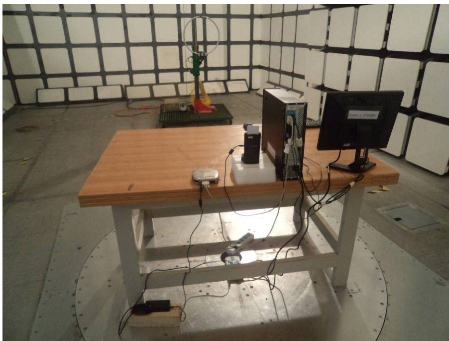
Radiated Emissions – Rear View (Below 30 MHz) (PC-Linked)
