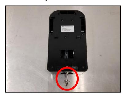
Unlocking the back-mount will cause it to disassemble into three parts: front cover, back cover, and the water-resistant part. Rubber adapters are also included inside the backmount.
