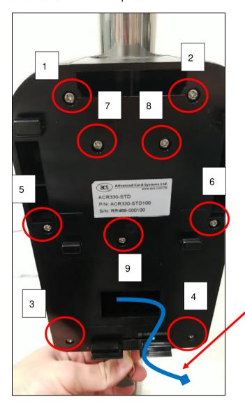
Note: This is where the Connection Cable (ie, Power Cord) will go through. Make sure that the cables are out so that they may be easily connected to the ACR350 Validator later on.
