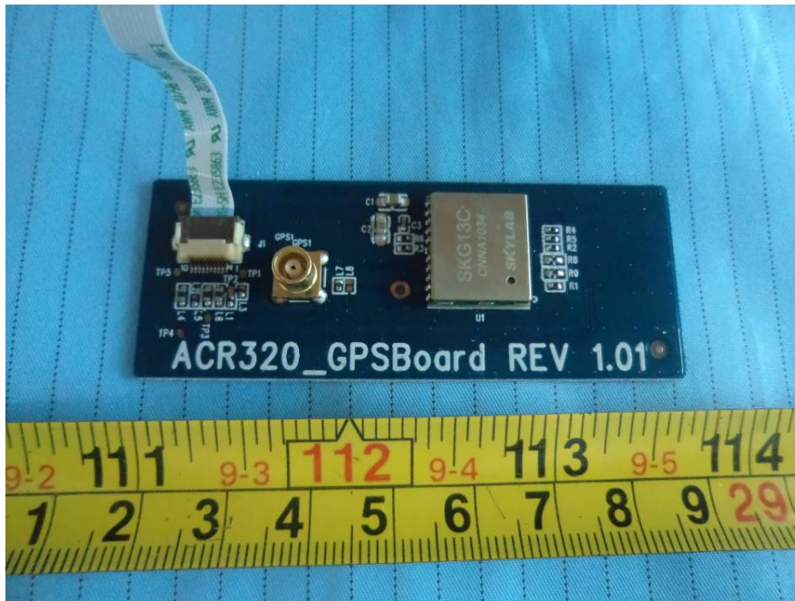
EUT – GPS Board Top View
